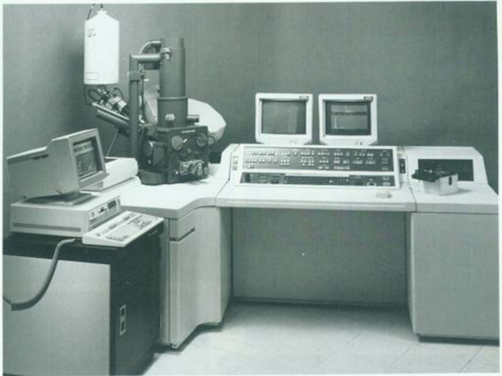
Figure 7-1(B) Photograph of a modern Cambridge SEM equipped to do x-ray analysis . (Courtesy of Leica.)
