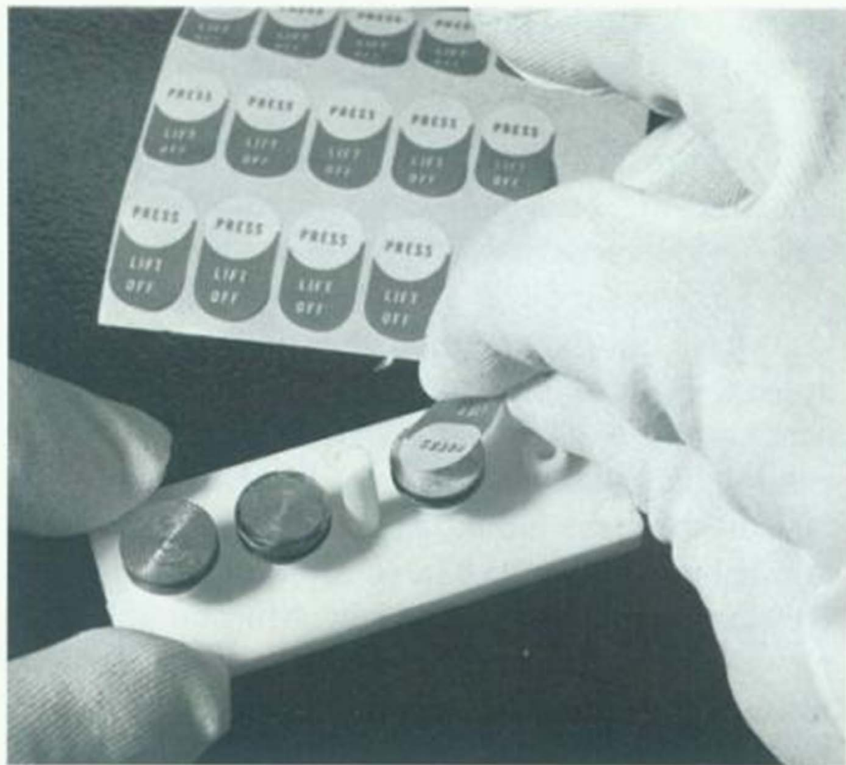
Figure 3-13 Adhesive transfer tabs are used to deposit a small amount of adhesive onto SEM stubs . The adhesive is adequate to hold most small specimens on the stub.
