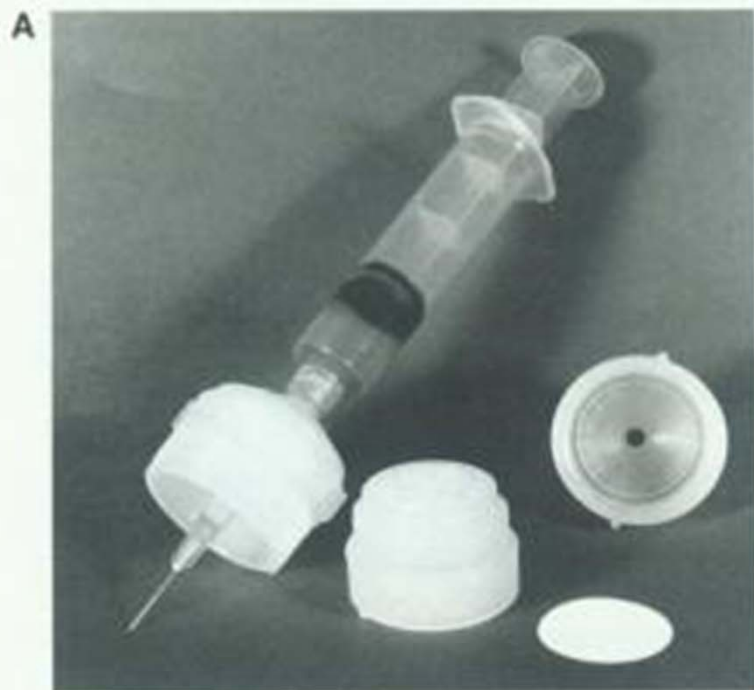
Figure 3-2 (A) Individual cells or tiny specimens suspended in a buffer system may be deposited onto microporous filters by passage through a filtering device, as shown. Fixatives are then syringed over the cells, followed by ethanolic dehydration. The filter holder is then opened, and the filter is removed, dried, and mounted onto a specimen stub. After
